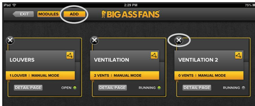
Figure 17—Adding and deleting louver/vent groups
