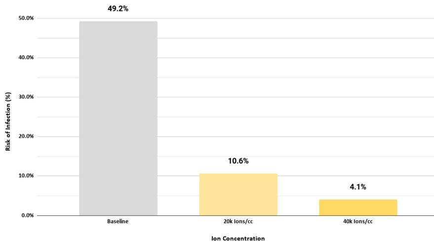
**Figure 3:** Wells-Riley Risk Reduction Estimate for 20k and 40k avg. ions compared to baseline mechanical systems in a sample office space.
