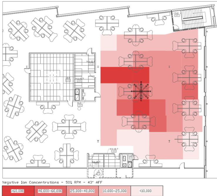
**Figure 2:** Ion concentration gradient at 50% RPM and 43" AFF.
