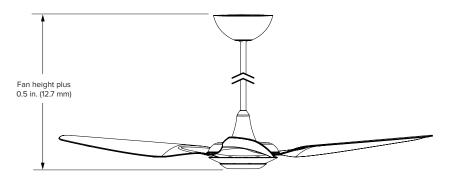
The Haiku Fan Light Kit adds 0.5 in. (12.7 mm) to the total fan height. See the Haiku fan spec sheet for exact fan heights, which depend on the fan's mount, diameter, and other factors.
