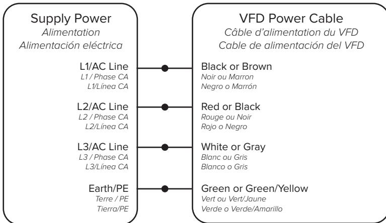
Connection to ungrounded 480 VAC Delta or Open Delta transformer secondaries should be avoided.
